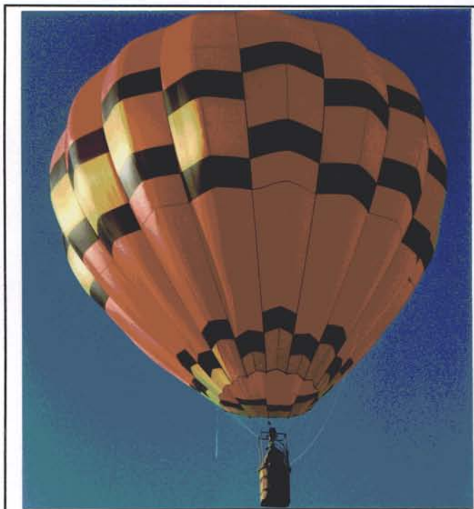
Figure 1. This 42,700 cubic foot envelope weighs 60 pounds, cost $1,261 and required 228 hours to design and build.
