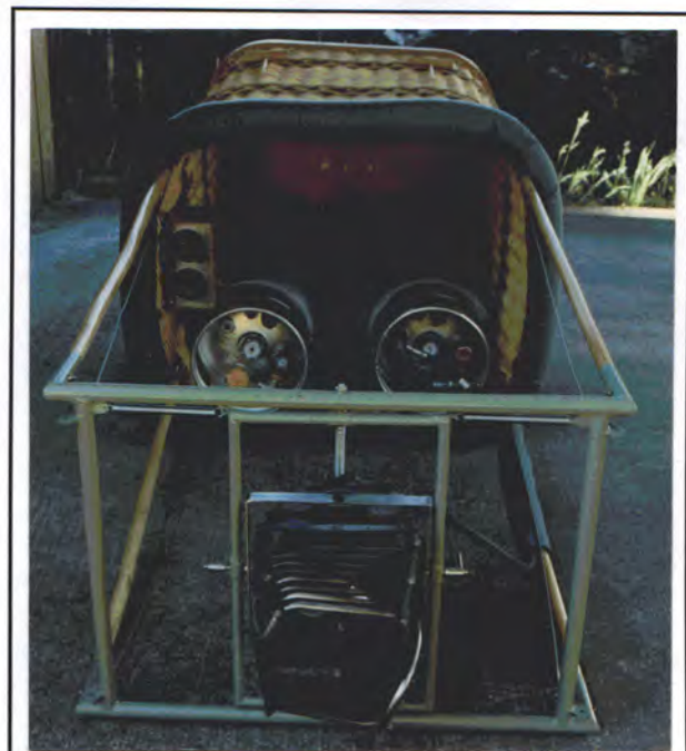
Figure 2: Looking into the basket, we see two Worthington ten gallon tanks and the instrument package. This photo was taken as part of the original airworthiness application. The burner is a Raven HP I, vintage 1978. This burner support ring was replaced after the second flight due to shortcomings described in the text.
