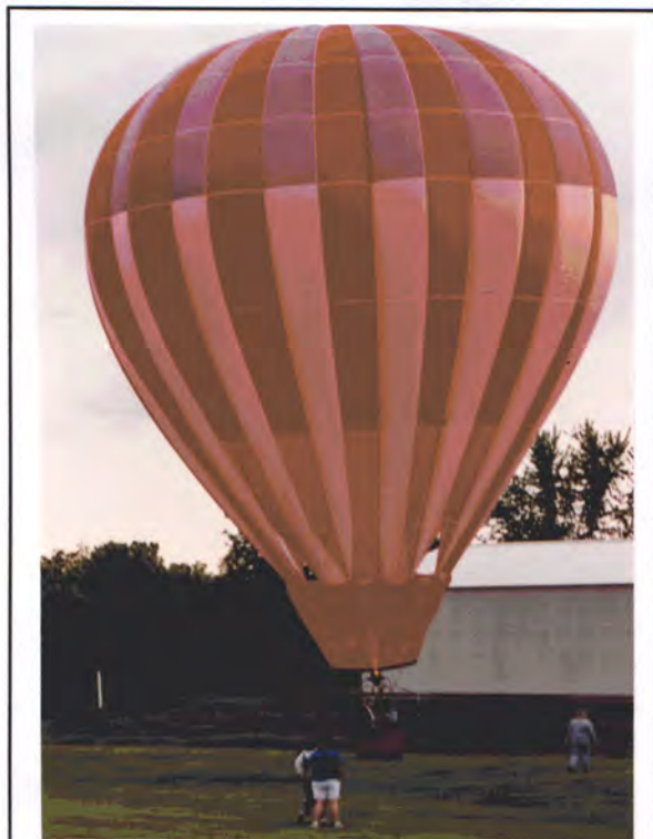
Peter Asp's homebuilt envelope based on an Aerostar S-52A gore pattern.
