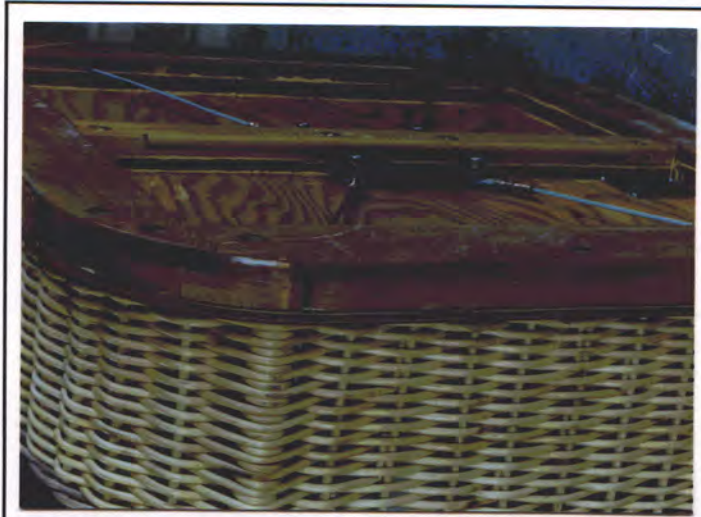
Figure 3: This view of the basket bottom shows the steel plate to which the basket support cables are attached. The glue lines clearly show the two wood layers which make up the basket skid assembly. The slot in the near side of the skid plates is to allow a replacement cable to be fitted to the basket without cutting apart the base.
