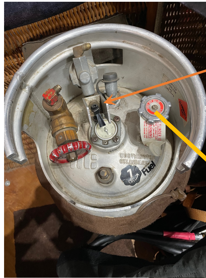
Liquid valve, angle globe type
